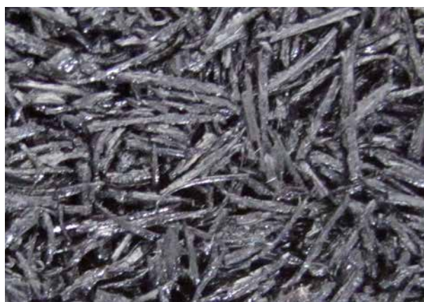
The material structure of our Regupol® Elastic Tiles RG is distinctly more open compared to our Regupol® Elastic Tiles.
